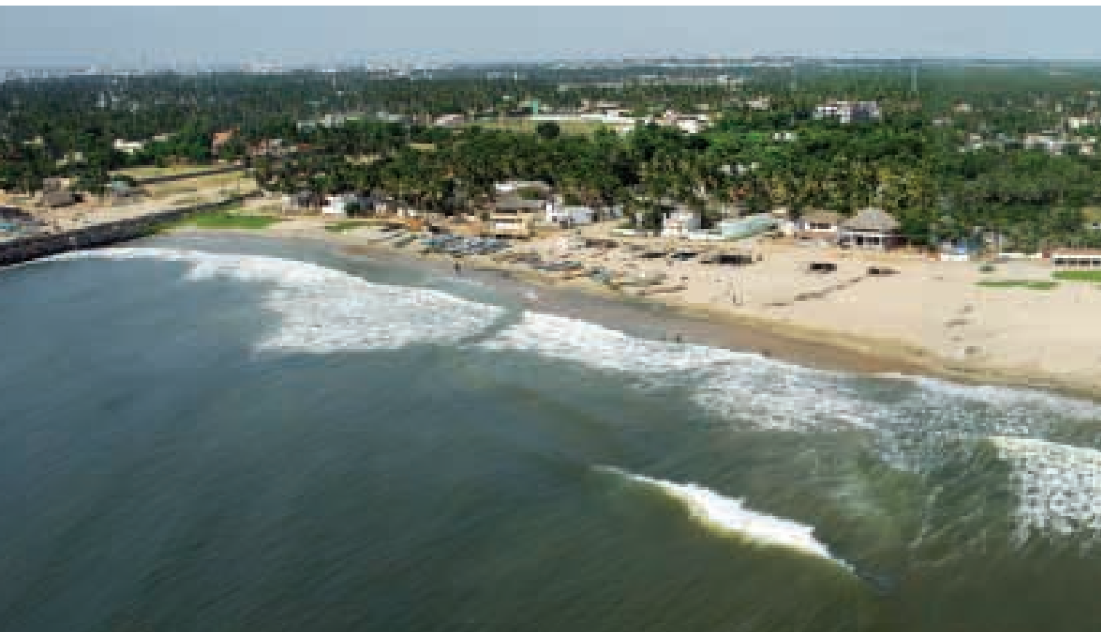
Figure 5.31: Disruption of littoral drift caused by groyne resulting in erosion. Aerial panoramic view of Banyan beach and groyne at Thandirayankuppam, 16 September 2012
