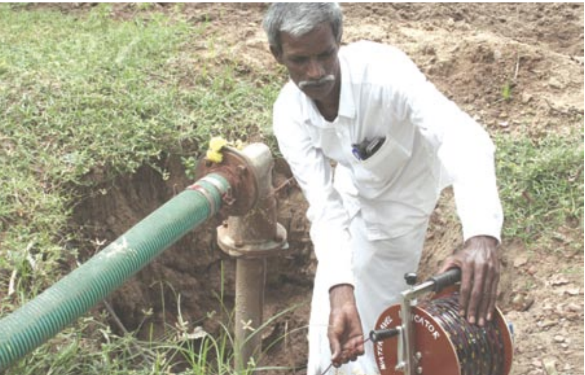
A simple tool: Water level indicator
