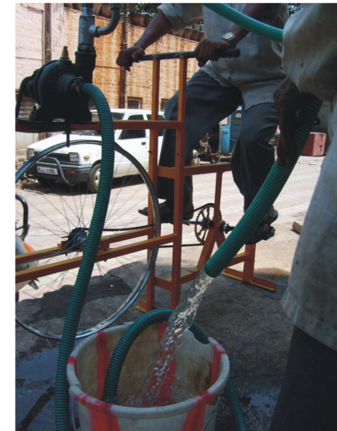
Water running through the delivery pipe.
