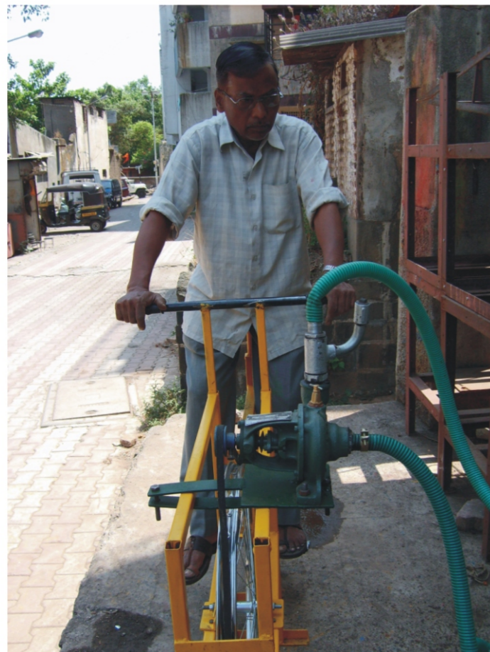
Peddling to operate the pump
