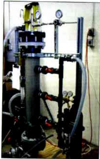
Figure 6.3: Advanced Nitrate Reduction Hollow-Fiber Membrane Bio-Reactor
