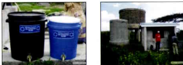
Figure 3.3: Eawag fluoride removal by bone char
