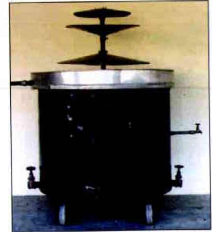
Figure 5.7: Water Iron Removal Unit of DRDO
