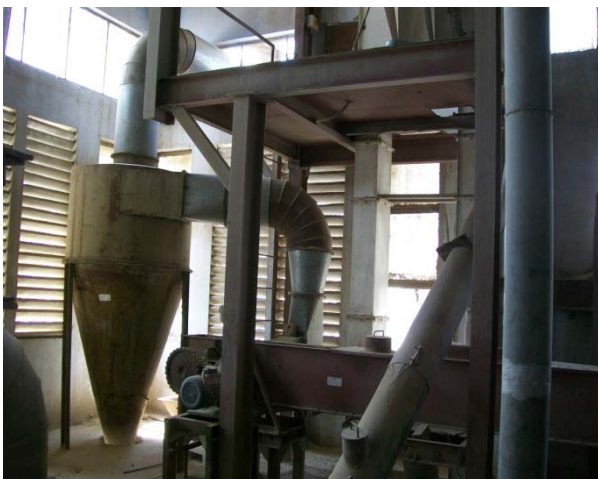
Fig 5.19-Proper dust extraction system with cyclone and ID fan in Large mills
