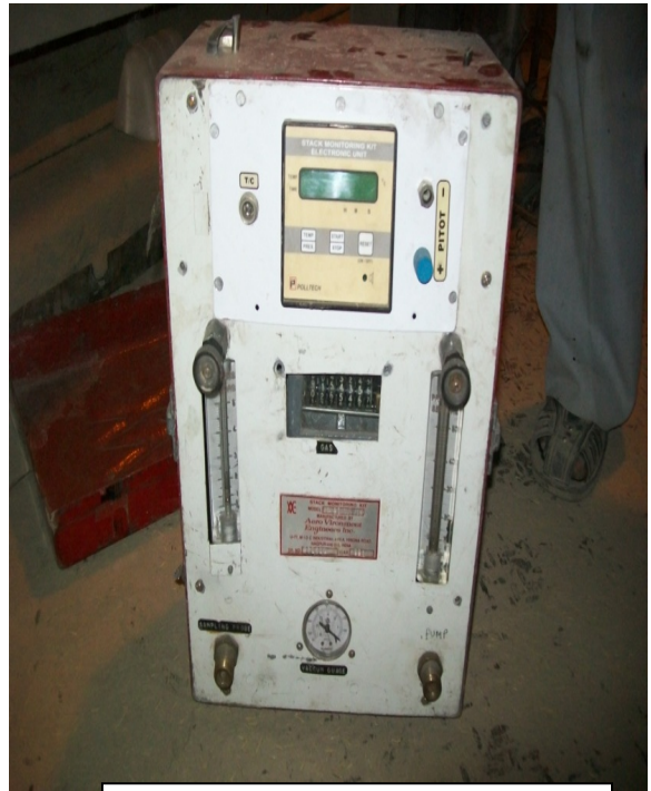
Fig. 6.2 Stack Monitoring Kit
