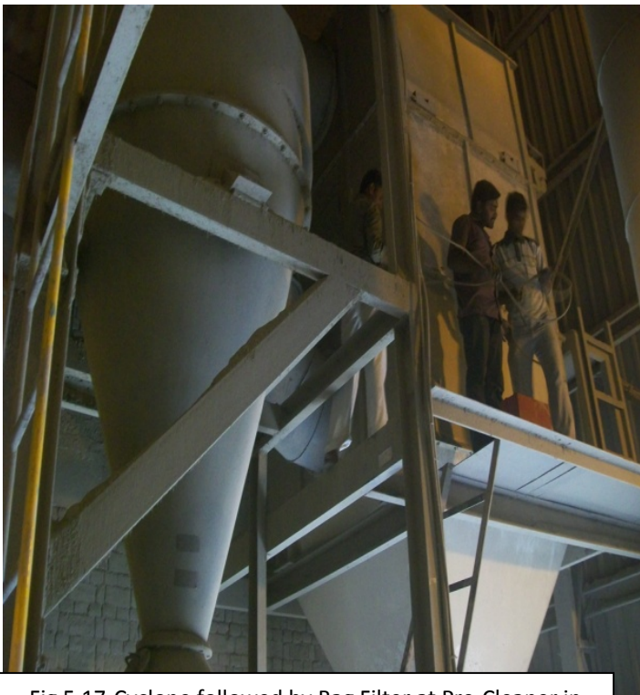
Fig 5.17-Cyclone followed by Bag Filter at Pre-Cleaner in large mills
