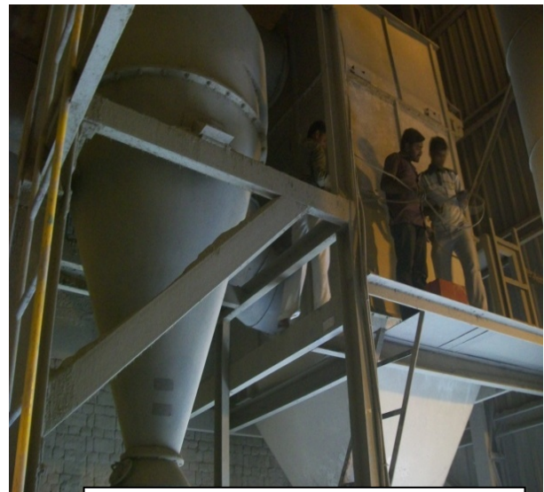
Fig.6.5 Cyclone followed by Bag Filter
