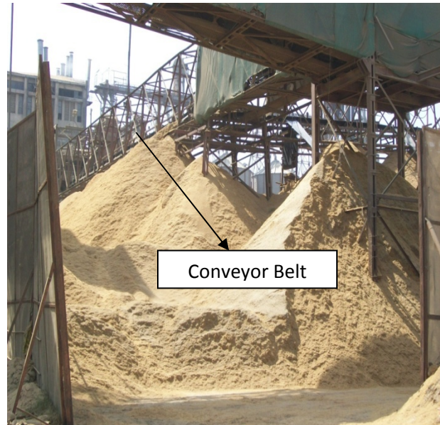
Fig 4.5-Rice husk conveyance in storage yard using conveyor belts
