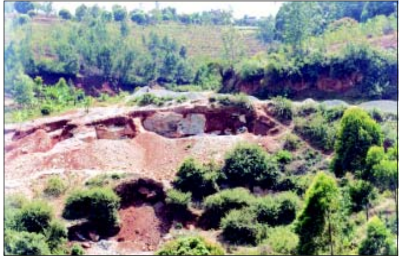
Plate 6. Stone quarrying in a peri-urban area. The loosened soil is washed by rain down the slope to the river where it is deposited as silt.
