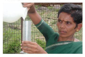
Daily rainfall measurement is collected from rain gauge stations distributed for every 5sq.kms in the project area. Rainfall Measurement is carried out by farmers themselves after establishing over 190 rain gauge stations in the project area spread over 65 drainage units.
