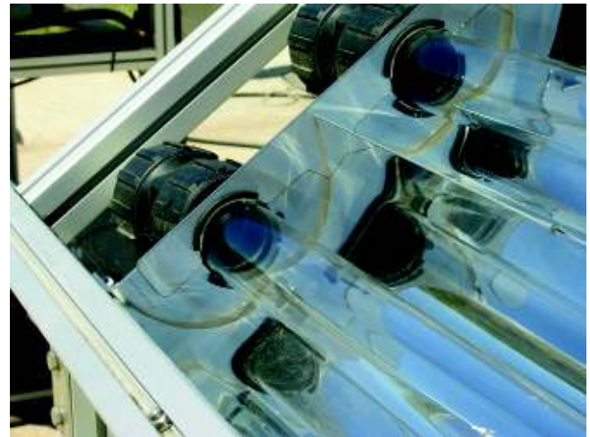
Fig. 8. Solar CPC reflector of anodised aluminium installed in a photo-reactor prototype made with glass tubes of 5 cm external diameter (picture taken at Plataforma Solar de Almería, Spain).
