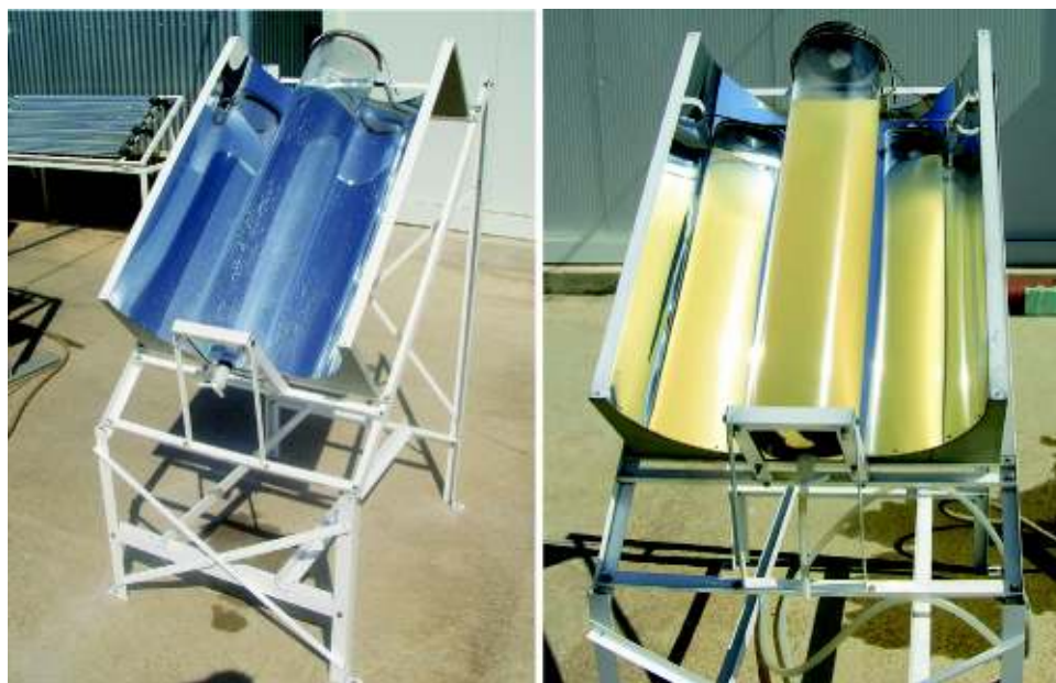
Fig. 9. SODIS enhanced batch reactor of 25 L containing water of 0 and 100 NTU (picture taken at Plataforma Solar de Almería, Spain) [49].
