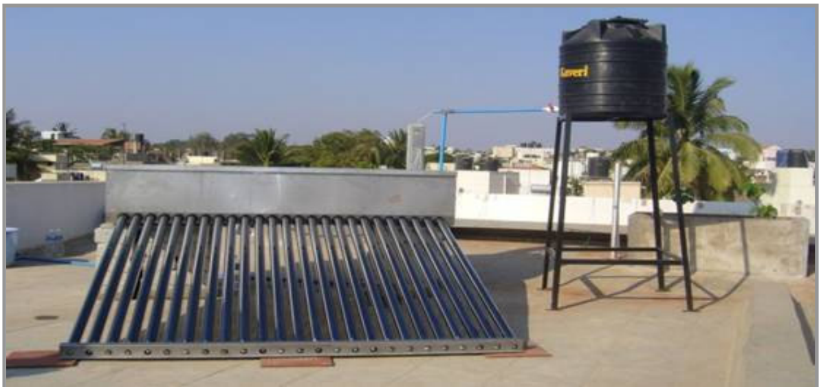
Prototype solar still under test in TERI premises, Bangalore; with vacuum tube collector
