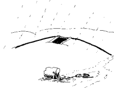
2. Mouth of hole built up to keep out runoff
