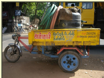
Removal of black water from septic tank in barrel mounted on tricycle
