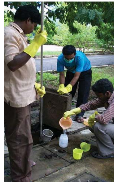
Wastewater collection from Anaerobic Filter
